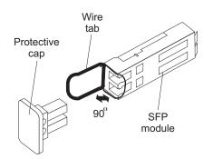
Figure 29. Unlocking the SFP module latch - wire variety
